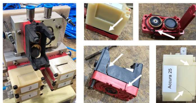
Figure 10. P8 valves after CC60 campaign.
